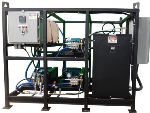
E3S425EA3-EK24144A-460 PCO50 12gpm@2500psi w/144kw heater & 50gal tank, PLC controlled
